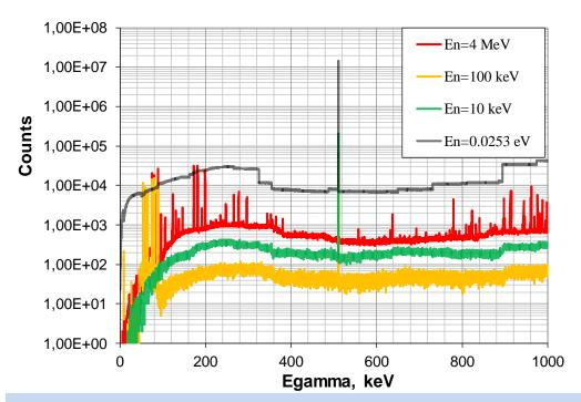
Spectra of the emitted gamma-quanta in metallic gadolinium with 2 mm thickness, irradiated with monochromatic neutrons in a broad energy range, simulated with GEANT4.
