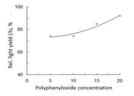
The dependence of the light output of PS I / I on the concentration of polyphenyl oxide (the diffusion amplifier in polystyrene) at the radiation dose of 2,8 Mrad. The introduction of diffusion amplifiers into the polymer base of a PS can lead to an increase in its radiation hardness.
