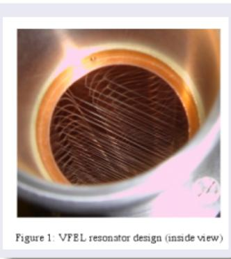
Figure 1: VFFEL resonator design (inside view)
