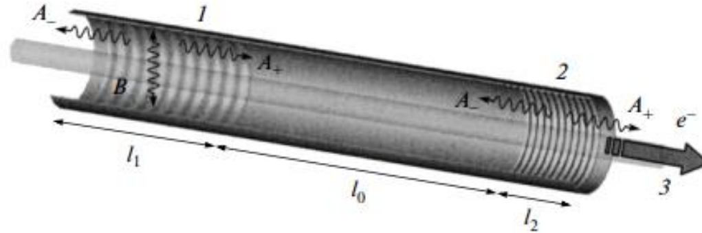
Fig. 1. Schematic diagram of a FEM with a combined double-mirror resonator: (1) modified Bragg reflector (2) traditional 1D Bragg reflector; (3) electron beam. Wavy lines show the directions of propagation of the electromagnetic flows A_{\pm} and B . The corrugation period of the modified Bragg structure (1) is about twice that of the traditional structure (2).
