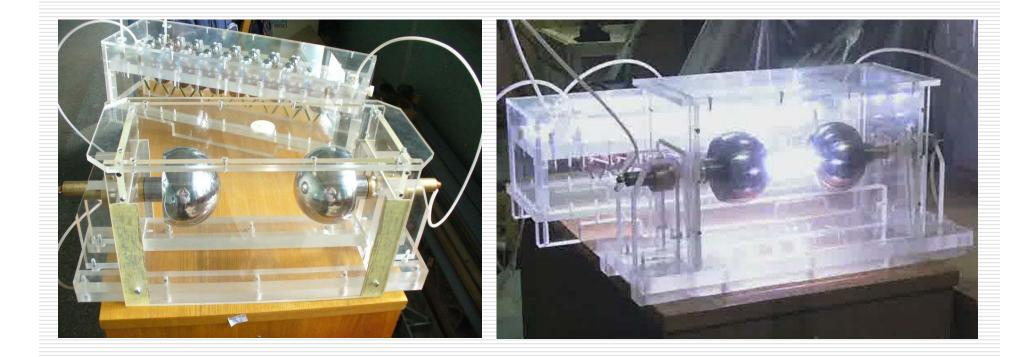
The output voltage of the Marx generator is measured by the accurate measuring discharge gap as high as 300 kV. The Marx generator rise-time is less than 50 ns.
