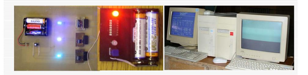
Test objects are the elements of analog and analog-digital dynamic circuits (for example, relaxation oscillator) specially developed for such experiments. LEDs in these circuits make circuit drop-in visible.
