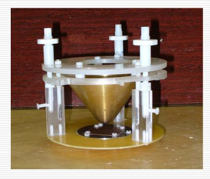
The cone with the angle 70° is made of brass and placed over the steel plate with the tungsten electrode.
