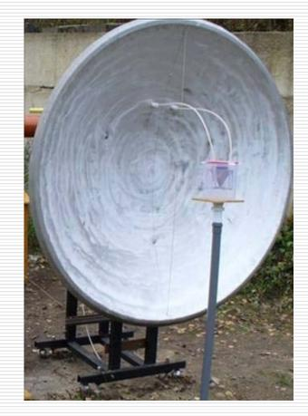
The antenna is placed at the focal point of the dish reflector 1.6 m in diameter. A convergent mirror is used for optimization of the antenna yield. The dish reflector and convergent mirror direct and amplify the signal from the antenna in the prescribed direction simultaneously keeping it off electromagnetic pulses from other sources (for example, discharge gaps of the Marx generator).
