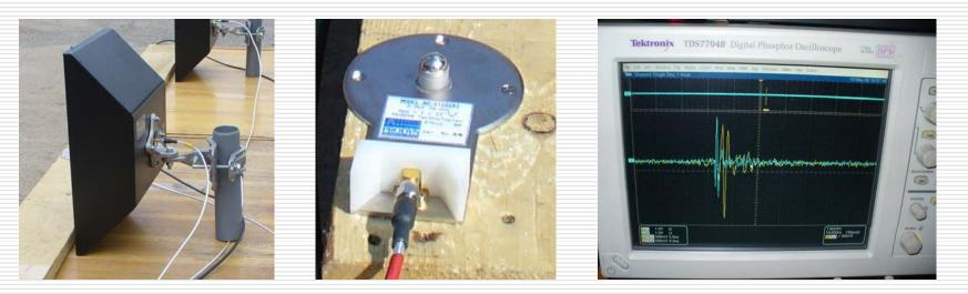
Measuring antennas Geozondas GZ031ANL-2 and D-dot Prodyn probes AD-S110(R) are placed as field probes at the distance 30 meters from the radiating antenna and connected to the Tektronix TDS7704B digital oscilloscope hidden in a shielded room and operated from an uninterruptible power supply.
