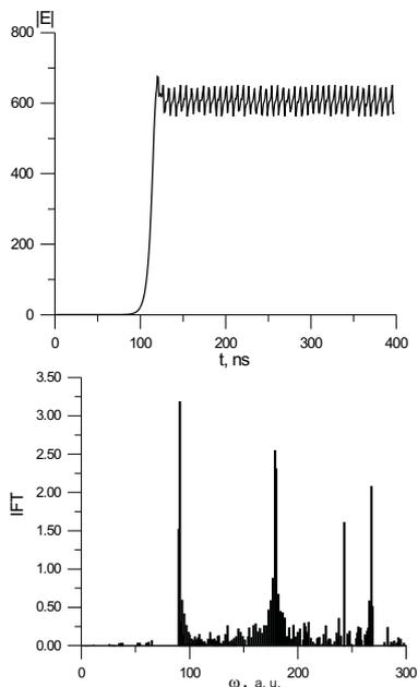
FIG. 3. Quasiperiodic regime (a) for transmitted wave and (b) its intensity Fourier transform
