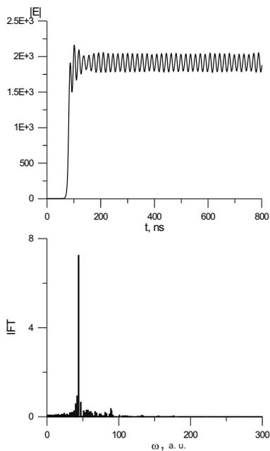
FIG. 2. Periodic regime (a) for transmitted wave and (b) its intensity Fourier transform
