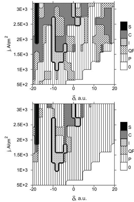
FIG. 8. Root to chaos (a) for transmitted and (b) diffracted wave. 0 means that the beam current is under threshold current. P – periodic regimes 1T, 2T etc. QP — quasiperiodicity. I — transition between two mode. C — weak chaos. S — stochastic self-oscillations.
