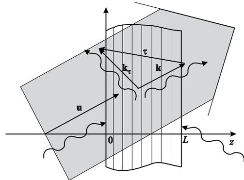
FIG. 1. Scheme of two-wave VFEL in Bragg geometry.
