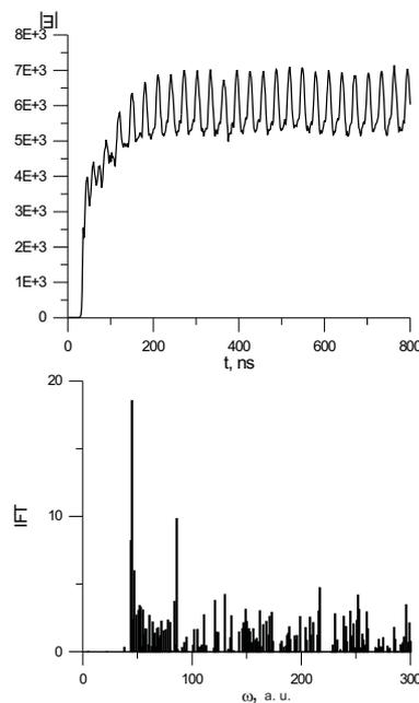
FIG. 4. "Weak" chaotic regime (a) for transmitted wave and (b) its intensity Fourier transform
