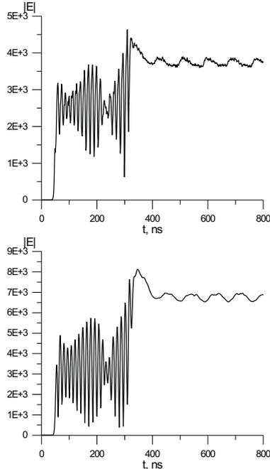
FIG. 7. Transition between two modes in VFEL (a) for transmitted and (b) diffracted wave
