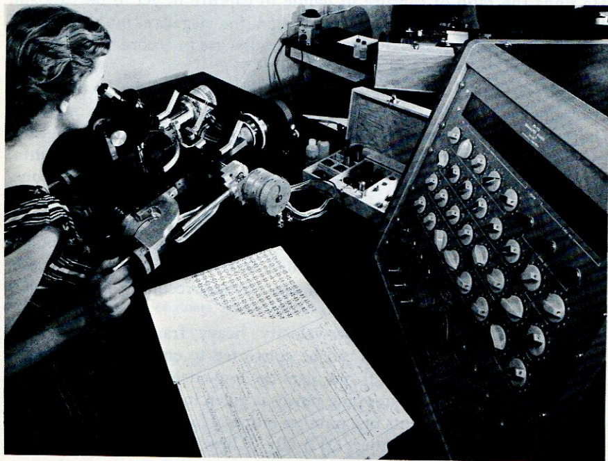
FIG. 10.9.2. Digitized Livermore scanning microscope and associated equipment. An enlarged section of the grid is helpful in plotting the paths of particles through emulsion pellicles. (Courtesy of R. S. White.)
