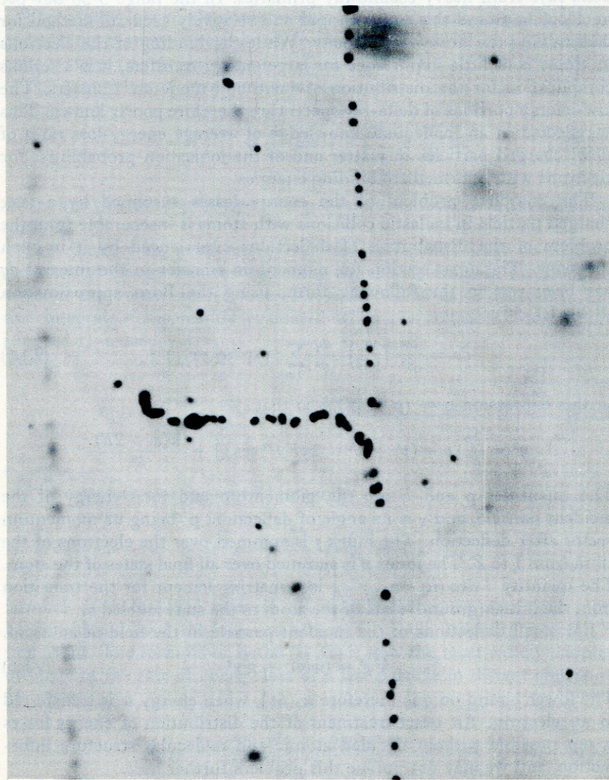
Fig. 9.1.5. Delta ray whose initial direction appears to indicate the direction of motion in the primary track. (Photomicrograph by C. Cole.)
