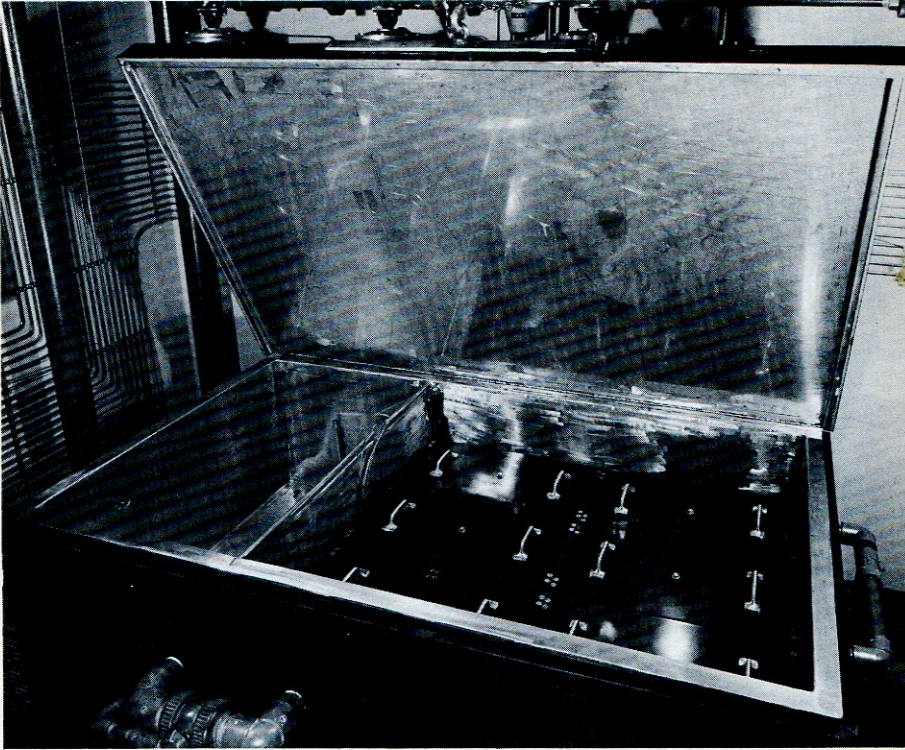
FIG. 5.4.3. View of main processing tank which is used for all the solutions (IDLRL).
