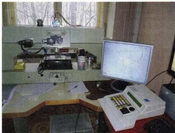
Fig. 3.27 Automated microscope PAVICOM-2 (FIAN, Moscow)
