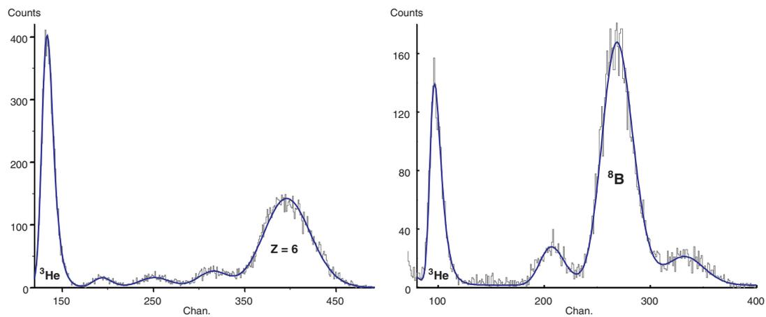
**Fig. 5.** Secondary beams produced by 2.0 A GeV/c  $^{12}\text{C}$  fragmentation at a beam line tune to the  $^9\text{C}$  fragment rigidity (left) and by 2.0 A GeV/c  $^{10}\text{B}$  at a tune to  $^8\text{B}$  (right).
