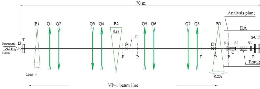
**Fig. 3.** Optical scheme of the beam line and detectors layout. Dashed marks (P) designate multiwire profilmeters. The S<sub>1</sub> counter of a diagnostic detector assemblage (EA) is placed close to a maximum position (analysis plane) of the beam line resolving function  $R(z)$ .
