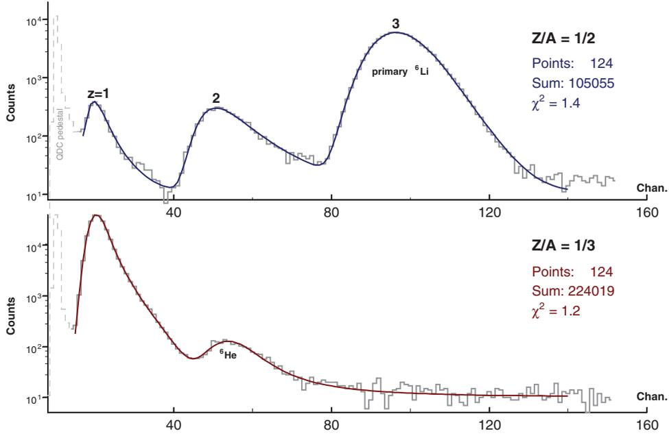
**Fig. 4.** Energy deposition spectra in a 8 mm scintillator registered in secondary beams produced out of 2.7A GeV/c  ${}^6\text{Li}$  nuclei interaction. Top: at beam line tune to rigidity of fragments with  $Z/A = 1/2$  (scale binding). The predominant peak **3** corresponds to the primary nuclei passed the target without interactions. Bottom: at  $Z/A = 1/3$ . Smooth curves are fits of type (3).
