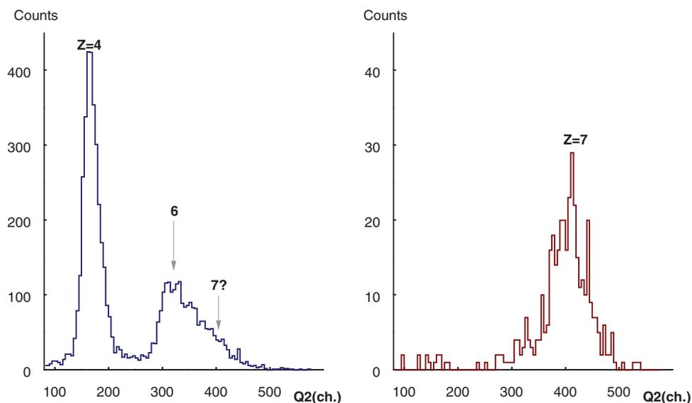
**Fig. 8.** Signal spectra of the 5 mm  $S_2$  analyzer. Left: a histogram of events with a TOF cut only vertical solid lines in the right plot of Fig. 7. Right: with an additional low limit cut on the  $S_3$  signal.
