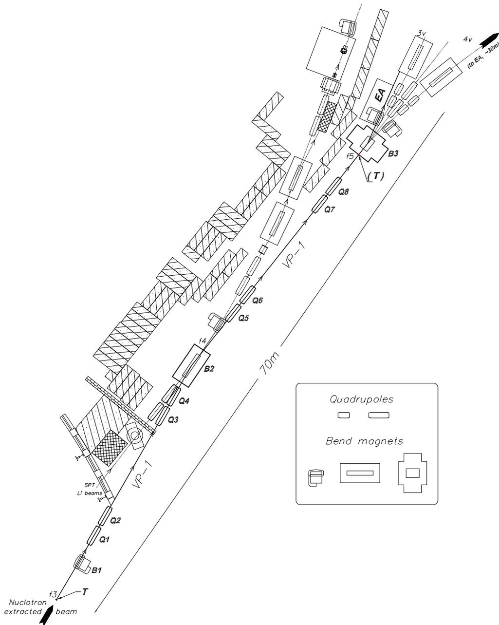
**Fig. 1.** Scheme of an experimental area at Nuclotron extracted beam. The main part of the VP-1 beam line and the 4v line were applied to form secondary nuclear fragment beams for emulsion irradiations. T – stripping target positions. EA – emulsion assemblage positions.
