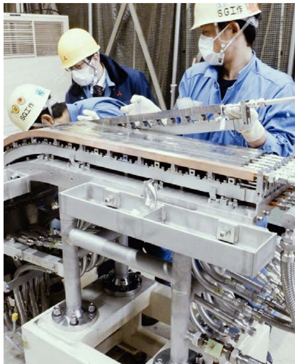
Plasma-facing units of the ITER divertor outer vertical target prototype have been mounted on a test assembly for high heat flux heating in Japan. The conditions at the bottom of the machine, where waste gas and impurities are exhausted from the reactor, can be described as extreme. Courtesy of ITER Organization.
