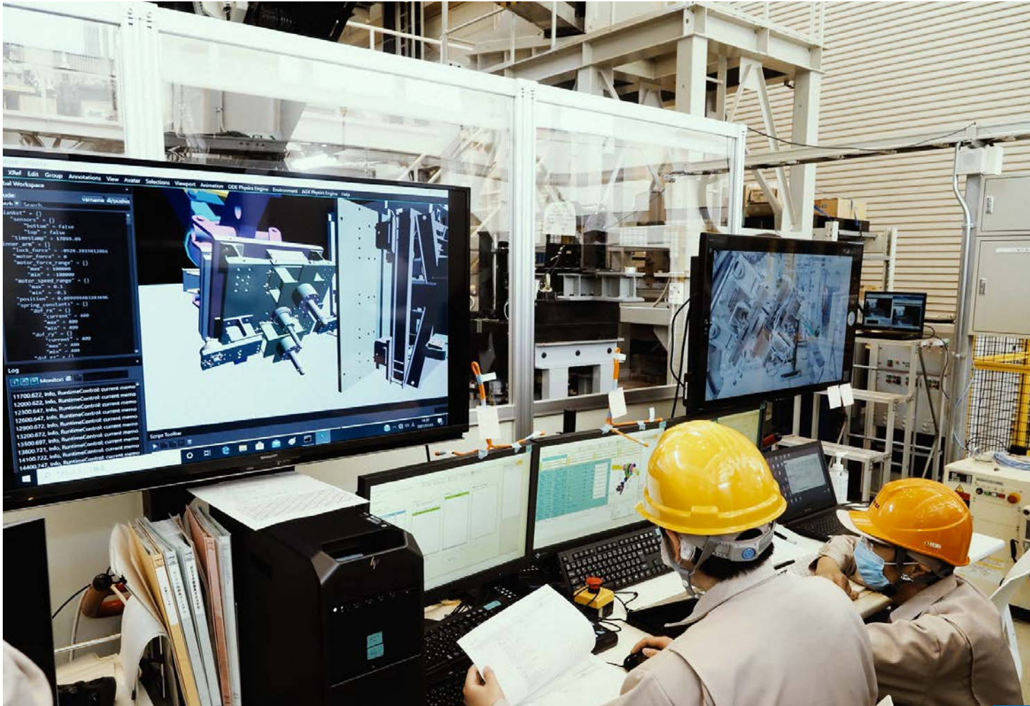
Engineers in Japan test a prototype of the control system for the ITER blanket remote handling system. On the left screen is a virtual reality model; on the right is the view from the camera. Look closely to see the manipulator on the other side of the window. Courtesy of ITER Organization.
