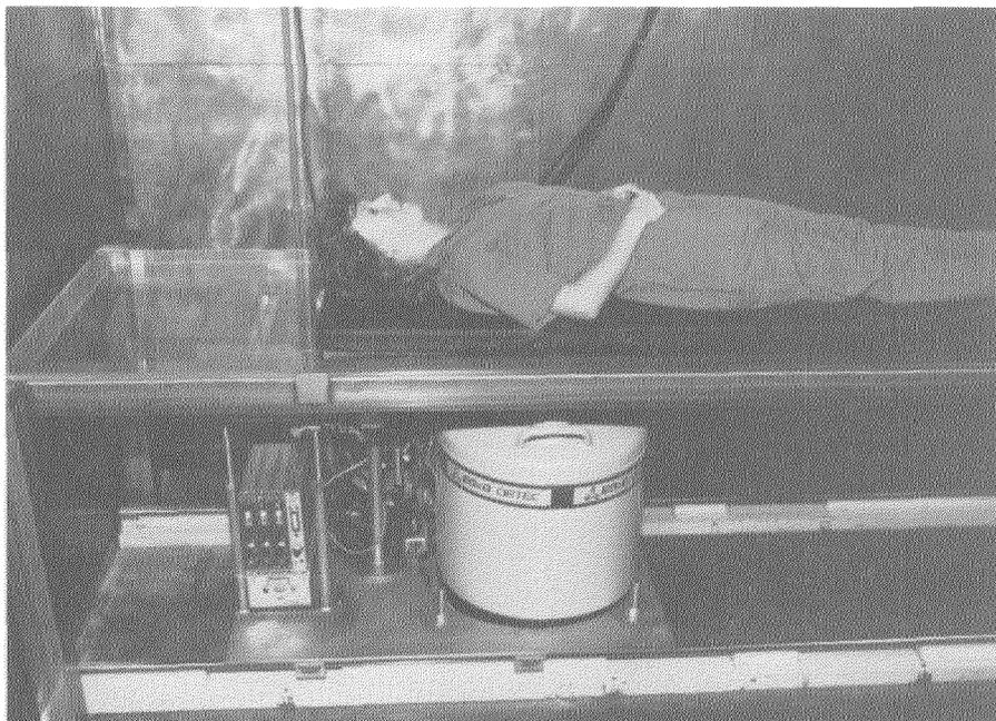
*FIG. IV-3. The four-detector array scanning the posterior surfaces of the supine subject in an investigation of internal  $^{60}\text{Co}$ .*
